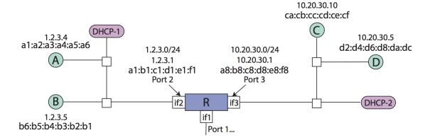
Consider the above topology. Here, two networks are connected through router *R*. *R* has three interfaces, each associated with a port, MAC address, IP address, and subnet.
